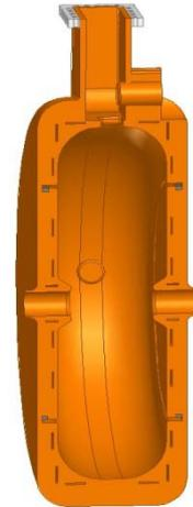
Fig. I-1.6.2: RF cavity with its harmful parasitic resonances damped.
